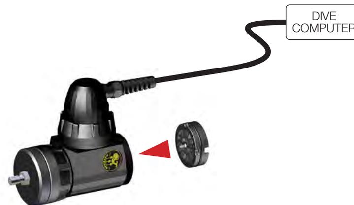
4. On the opposite end of the POD instal the mushroom valve with the membrane facing out, so that pure oxygen pressure can escape from inside the POD and no air can get in.
